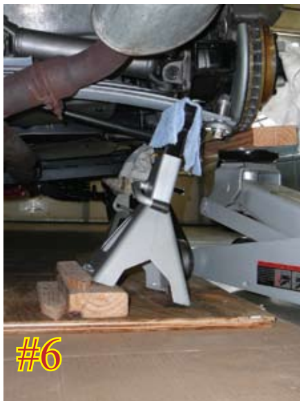
Close-up photo showing the position of the jack stand under the end of the leaf spring. Note that the vertical axis of the jack stand is close to perpendicular to the arch of the spring. This photo shows the stage of the process after removal of the link bolt, with the new retainer cup in place and with the swaging tooling in place ready to perform the swaging step.
