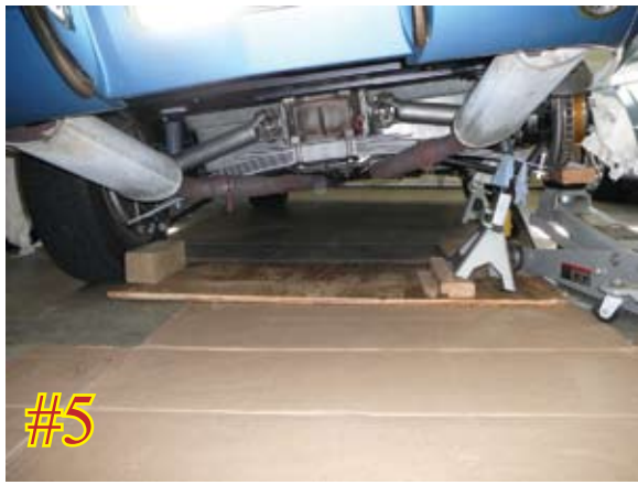
Plywood and blocking system in position to allow removal and replacement of the retainer cups on the passenger's side. The sequence of steps leading up to the stage shown in this figure is explained in detail in the text.
